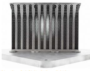
Intercooler on the build plate showing mesh detail
