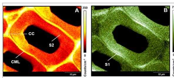
Figure 1. Raman images of cross section of Scots pine wood showing intensity changes of Raman band at  $1595\text{ cm}^{-1}$  (A, Lignin) and the orientation sensitive cellulose band at  $1095\text{ cm}^{-1}$  (B, Cellulose).
