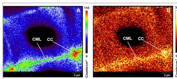
Figure 2. Raman images of cross section of decayed Scots pine wood showing A - lignin concentration changes (intensity changes of Raman band at  $1595\text{ cm}^{-1}$ ), and B - the increased concentration of pinosylvins (Raman band at  $1634\text{ cm}^{-1}$ ).
