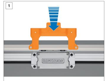
Place the setting shim between the readhead and the extrusion.
