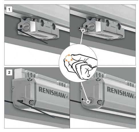
Removal of the air supply bung and fitment of the air connection fitting into either the readhead (1) or extrusion end cap (2). Finger tighten (0.3 Nm maximum).
