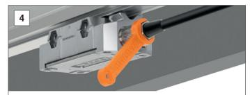
Using the included cable connection wrench with the hexagonal nut "B", secure the encoder cable.
