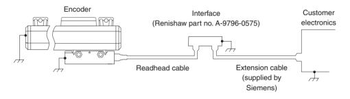
**NOTE:** On Siemens DRIVE-CLiQ systems the connector between the readhead cable and extension cable will mate via the A-9796-0575 interface.
