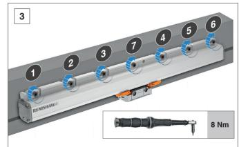
Using the correct tool, tighten the screws to a torque of 8 Nm. Tighten all bolts, working from left to right.
