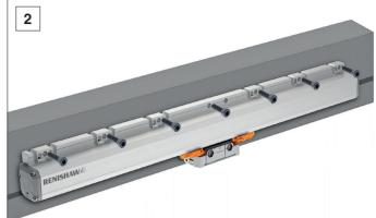
Loosely secure the extrusion to the mounting surface using M6 screws and washers as specified in section 12.3 on page 21.
