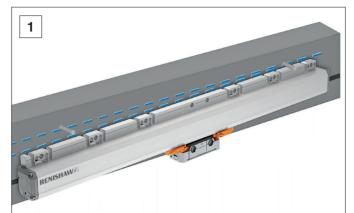
Place the encoder on the mounting surface and firmly push against mounting edge/dowel pins. Position the encoder to align mounting holes.
