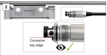
Insert the cable into the readhead. Take care to ensure correct connector orientation: the connector key edge should face towards the base of the readhead.
