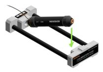
2. Extend the device so that the opposite end of the strut reaches the opposite ball surface of the calibrator. Ensure the RCS L-90 strut is magnetically attached to the calibrator.
