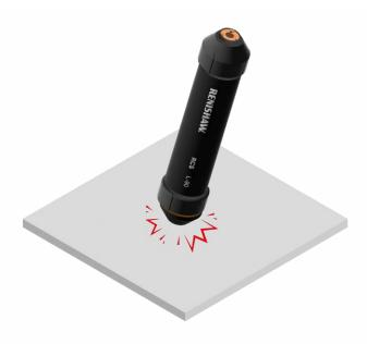
**IMPORTANT:** Any automated (robot-driven) compression beyond the RCS L-90 strut minimum length will require the offset to be recalibrated with the calibrator.
