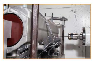
On-machine gauging using the RMP600
