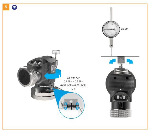
Tighten the opposing grub screws **3** against a locating pin fixed to the base.
