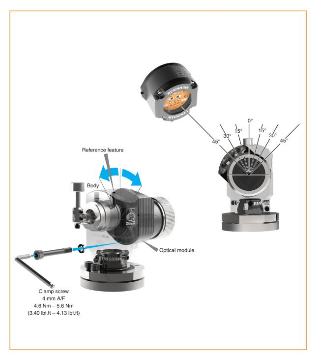
The optical module can be set in one of seven positions at 15° increments, to allow the optical window to point towards the receiver.
