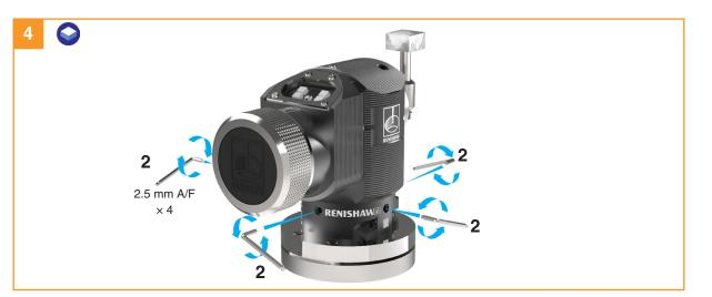
Slacken the four body locking screws 2.
