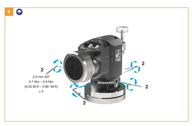
Fully retighten the four body locking screws 2.
