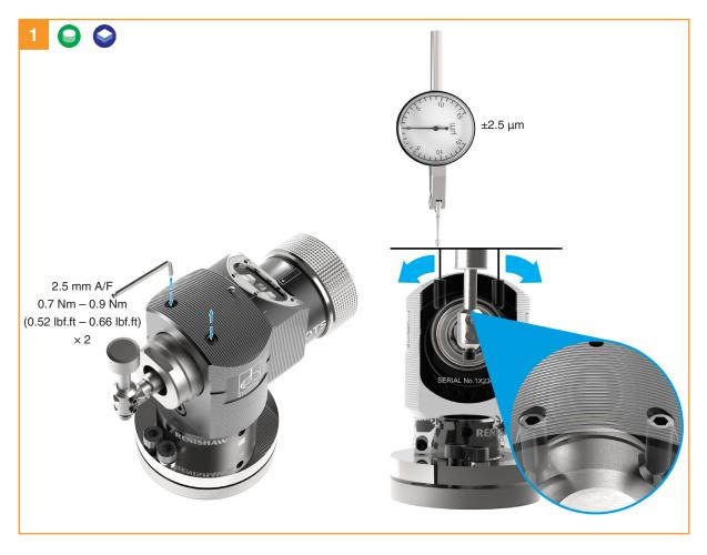
Side-to-side level adjustment is obtained by alternately adjusting grub screws, which causes the probe module to rotate and change the stylus level setting.
