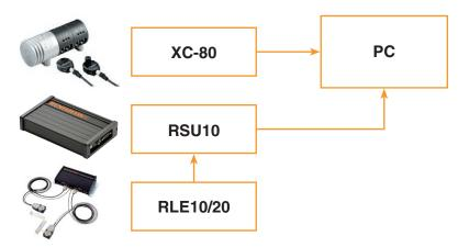
The RSU10 and an XC-80 can then both be connected to the PC via USB link. The compensated position can be viewed on standard Renishaw calibration software or on custom built software by use of the laser USB software development kit supplied with the RSU available from Renishaw.
