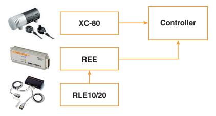
Again, since the XC-80 was designed for use in a calibration system it does not provide compensation in real time, the sensor readings will be updated once a minute. This is also reliant on the correct functionality exisiting within the controller.
