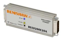
The REE will then produce a digital output, the resolution of which will depend on the type of REE. The output of the REE should then go directly to the RCU10 input.
