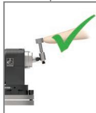
Deflect the stylus for 20 seconds until the status LEDs start to flash yellow eight times.
