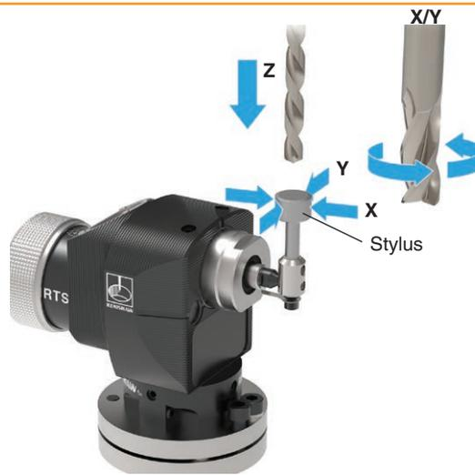
The tool is driven in the machine Z axis for tool length measurements and broken tool detection.
