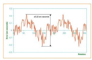
The total installed accuracy of a typical REXM system is  $\pm 0.22$  arc second, determined by analysis of sequentially rotated installations.
