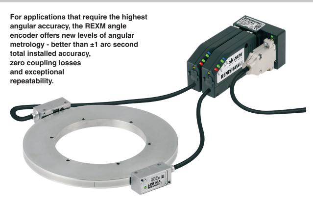
Like the RESM, the REXM stainless steel ring has graduations marked directly onto the periphery. However, it features a thicker cross-section designed to minimise all installation errors except eccentricity.
